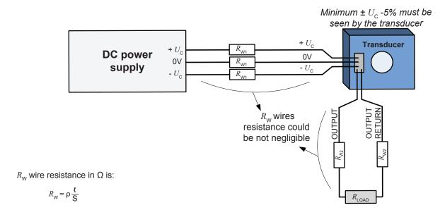
S: Cross section of wire in m<sup>2</sup>
